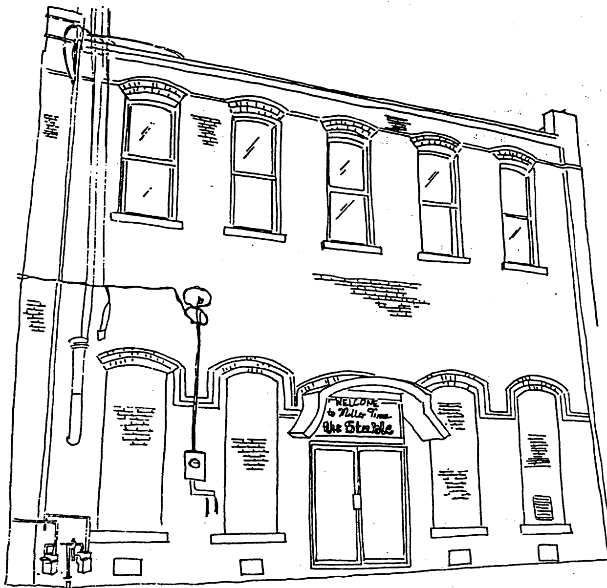
In addition to the signage, appropriate windows in openings and an awning at the entrance would further enhance this rear facade (300 block S. Lindell).
