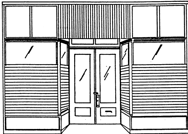
Transoms and display windows should not be covered or enclosed.
